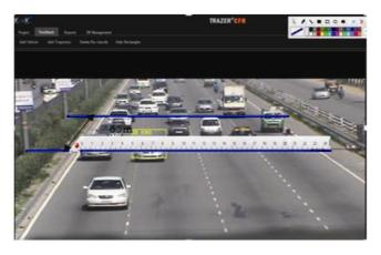
Figure 4. Entry and exit lines marked with screen marker and WINDOW RULER used to measure distance across width.
