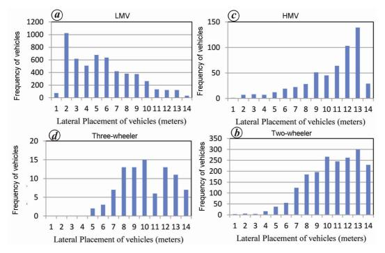
Figure 6. Frequency of vehicles across road width based on their lateral position for (a) light motor vehicle, (b) two-wheeler, (c) heavy motor vehicle and (d) three-wheeler.
