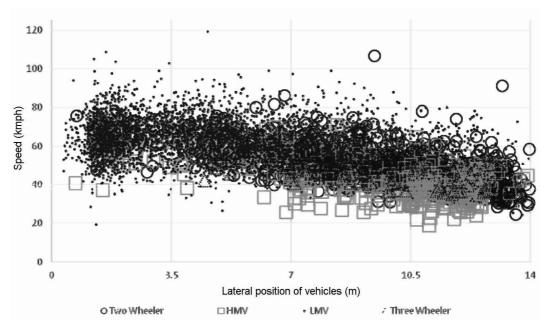
Figure 11. Variation in individual vehicle speed with lateral placement for all vehicle categories.
