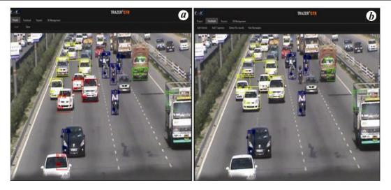
Figure 7. Vehicle detection with (a) default settings and (b) modified settings in TRAZER.
