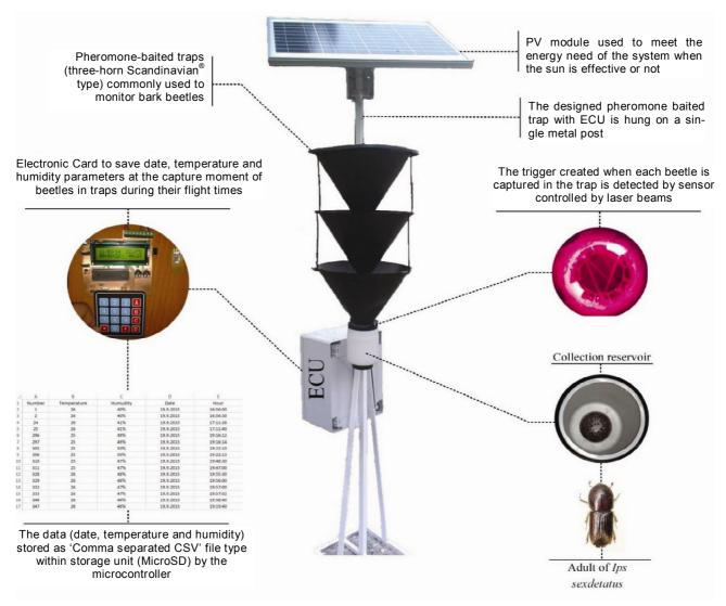
Figure 1. Design of prototype electronic control unit and system equipment.
