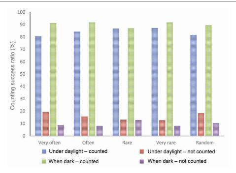
Figure 3. Counting success ratio depending on throwing frequencies under different light conditions of the ECU.
