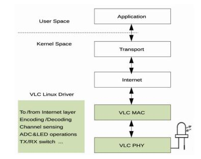
Figure 2. Communication stack of VLC in an embedded Linux operating system.
