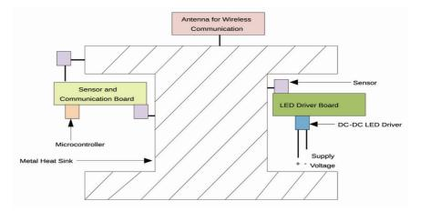
Figure 1. Visible light communication module.
