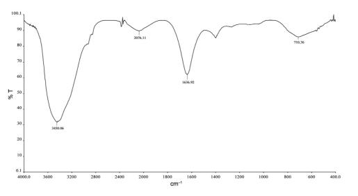
Figure 2. FTIR spectrum of red soil after addition of graphite.
