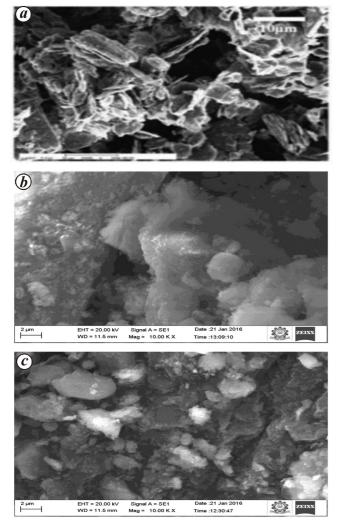
Figure 3. SEM images of (a) graphite powder, (b) red soil sample and (c) graphite-added red soil sample.
