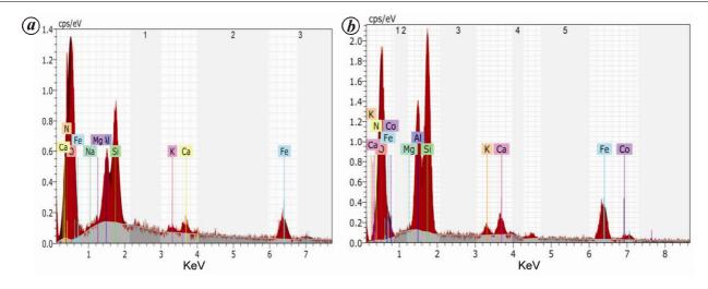
Figure 4. EDX images of (a) red soil sample and (b) graphite powder-added soil sample.
