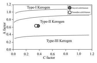
Figure 4. A factor versus C factor plot of Panandhro and Neyveli solid bitumen.
