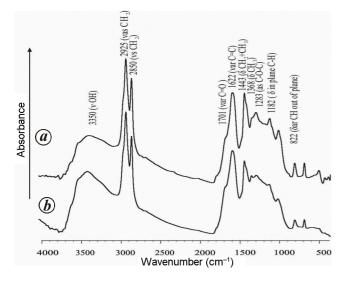
Figure 3. FTIR spectra of solid bitumen from (a) Panandhro lignite mine and (b) Neyveli lignite mine.
