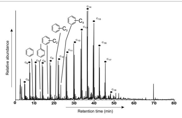
Figure 5. Pyrolysis mass chromatogram of Panandhro solid bitumen, Kachchh Basin (black dots indicating n-alkanes).
