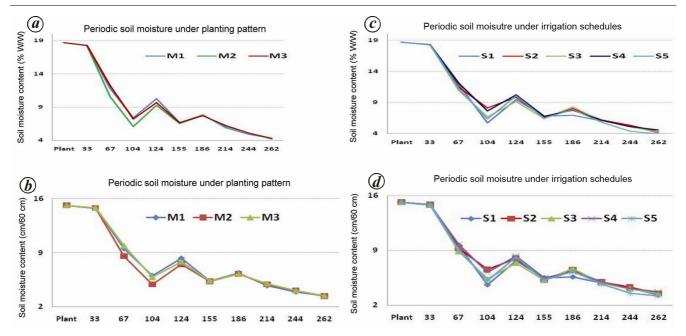
Figure 3. Trend in periodic (day) soil moisture (% w/w in surface soil and cm/60 cm soil profile) under different planting configurations and drip-fertigation schedules. M1, M2 and M3 are planting configurations and S1, S2, S3, S4 and S5 are drip-fertigation schedules as described in materials and methods.
