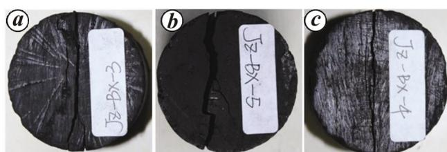
**Figure 9.** Splitting failure patterns of coal. *a*, Bedding parallel to disk surface; *b*, Bedding angle 90°; *c*, Bedding angle 0°.
