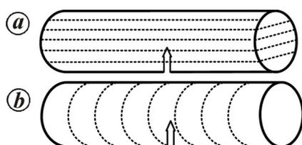
**Figure 10.** Relative position of incision plane and bedding. *a*, Incision plane perpendicular to bedding; *b*, Incision plane parallel to bedding.
