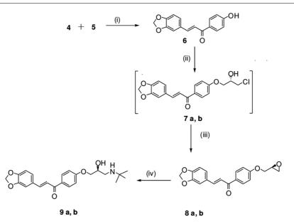
Reagents: (i) 20% aq. NaOH, MeOH, r.t., (ii) S-epichlorohydrin or R-epichlorohydrin, 100-120°C, (iii) aq. NaOH, PTC, toluene, (iv) t-butyl-amine, MeOH, r.t.
