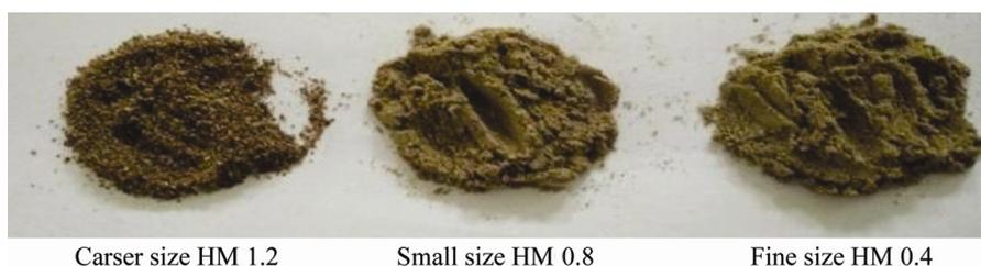
**Figure 1.** PNF of different size sample obtained from hammer mill HM 1.2, HM 0.8 and HM 0.4.
