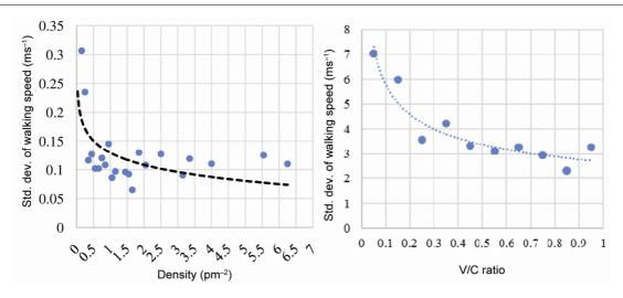
Figure 3. Variation in speed with increase in density and V/C ratio.
