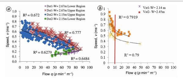
Figure 2. Flow-speed relationship: *a*, suburban station; *b*, interstate station.
