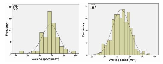
Figure 5. Frequency distribution of walking speed at different density regions for suburban station. a, Density <0.45 pm<sup>-2</sup>; b, Density >0.45 pm<sup>-2</sup>.
