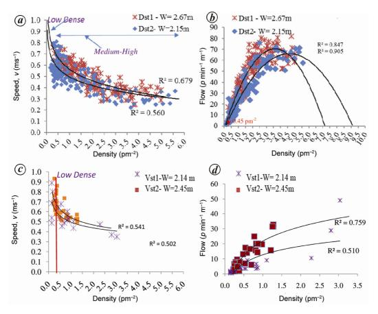
Figure 4. Fundamental relationships (a and b) for suburban and (c and d) for interstate station.
