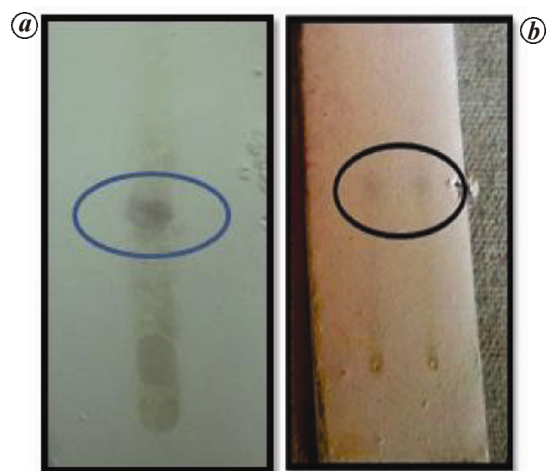
Figure 1. TLC chromatogram of (a) active sub-fraction (437–448) and (b) isolated compound, derivatized with NaOH-lead acetate solution, showed compound of interest (in circle).
