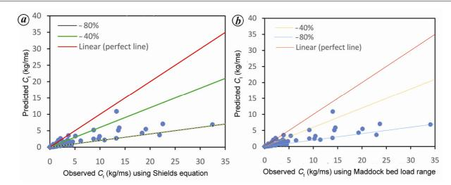
Figure 2. Percentage error between observed and predicted total load transport using (a) Shields' equations and (b) Maddock's range as bed load for Yang approach<sup>24</sup>.
