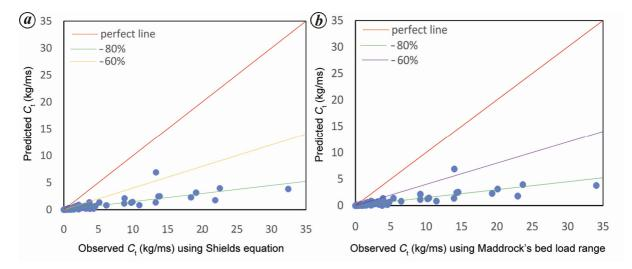
Figure 3. Percentage error between observed and predicted total load transport using (a) Shields' equations and (b) Maddock range as bed load for  $Yang^{25}$  approach.
