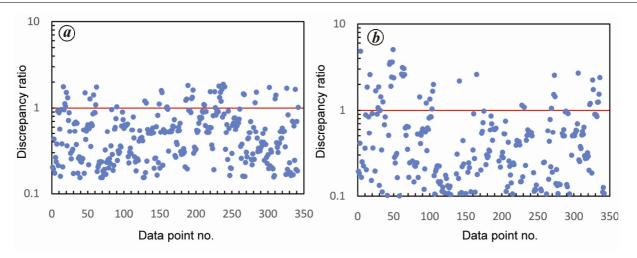
Figure 4. Verification of  $Yang^{24}$  Unit Stream Power for Shetrunji River data using (*a*) Shields' bed load formula and (*b*) Maddock's bed load range.
