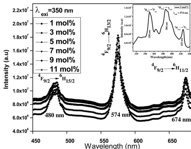
Figure 3. Emission spectrum of LaOF : Dy<sup>3+</sup> (1–11 mol%). (Inset) excitation spectra of LaOF : Dy<sup>3+</sup> (3 mol%).
