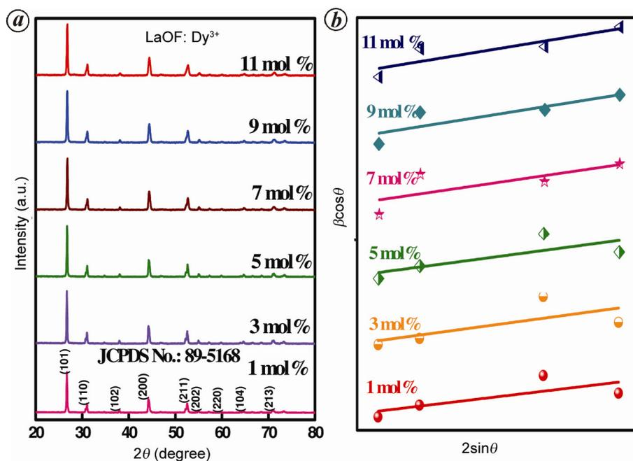
Figure 1. (a) PXRD pattern and (b) W–H plot of LaOF : Dy<sup>3+</sup> (1–11 mol%).
