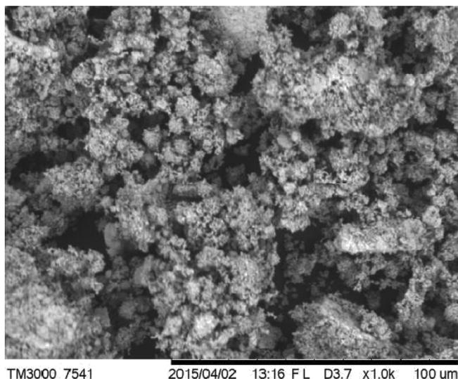
Figure 2. SEM image of LaOF : Dy<sup>3+</sup> (3 mol%).
