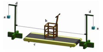
Figure 1. Test rig to measure dynamic push-pull strength capabilities. a, Varying load; b, four wheeled cart; c, treadmill; d, supporting stands.
