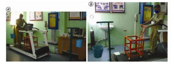
Figure 3. Performance on developed test rig. *a*, Push force; *b*, pull force.
