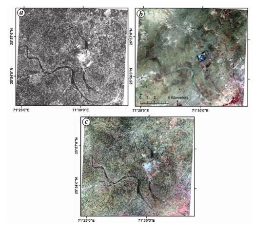
Figure 4. (a) Palaeochannels detected on RISAT-1 image in parts of Barmer, Rajasthan. (b) Corresponding Landsat OLI FCC image, and (c) optical and SAR-merged FCC. In optical and merged images, FCC is generated using combinations of bands 5, 4 and 3.
