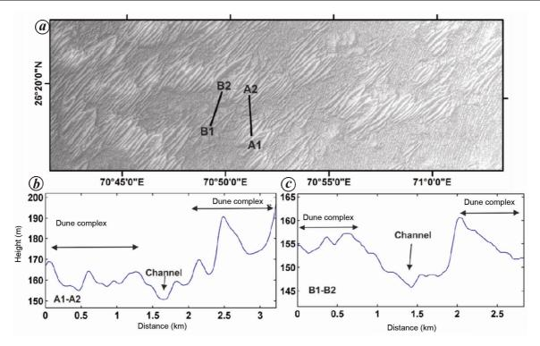
Figure 3. (a) Cartosat DEM covering southern parts of Jaisalmer district, Rajasthan and topographic profiles A1-A2 (b), and B1-B2 (c).
