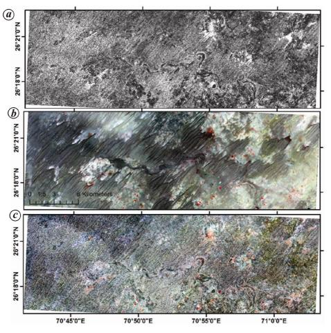
Figure 2. a, Palaeochannels detected on RISAT-1 image in the southern parts of Jaisalmer district, Rajasthan. b, Corresponding Landsat OLI FCC; c, Optical and SAR-merged FCC. In optical and merged images, FCC is generated using combinations of bands 5, 4, 3.
