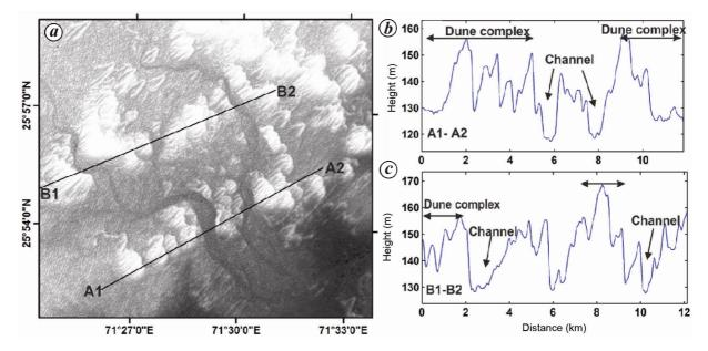
Figure 5. *a*, Cartosat DEM covering parts of Barmer district, Rajasthan. Topographic profiles A1–A2 (*b*) and B1–B2 (*c*).
