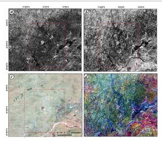
**Figure 6.** a, Feeble pattern of palaeochannels seen on RISAT-1 HV image, west of Pachpadra playa, Barmer district. b, Enhanced palaeochannels in RISAT-1 HH image. c, Corresponding Landsat ETM FCC showing feeble pattern of main channel only. d, Radar and optical merged image using PCA technique enhances the palaeochannels.
