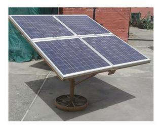
Figure 2. Solar photovoltaic panel for operating the cooling system of SPOSS.
