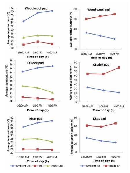
Figure 4. Hourly variation of temperature and relative humidity for ambient and inside the SPOSS.
