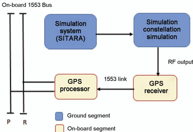
**Figure 11.** Test set-up with GPS RF simulator.
