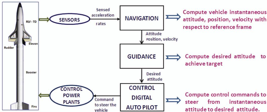
Figure 1. Functional diagram of navigation, guidance and control system.
