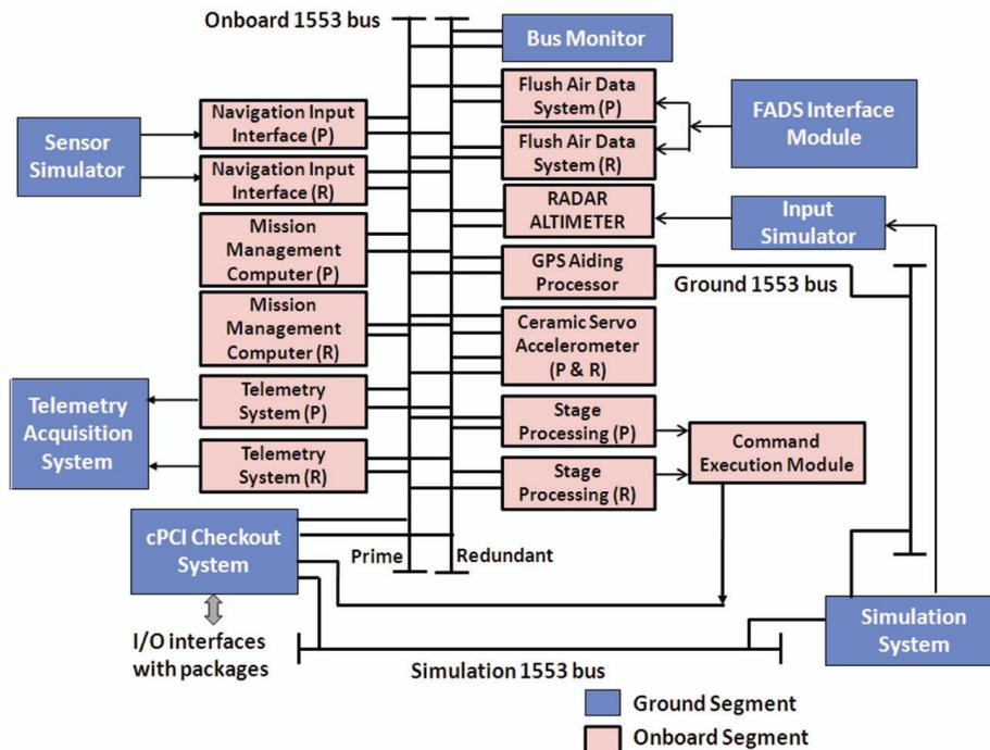
Figure 6. Block schematic of OILS test bed.
