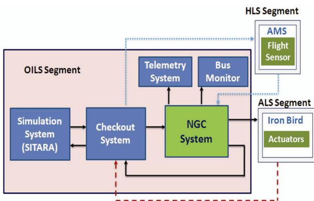
Figure 5. Block schematic of NGC test-bed configuration.
