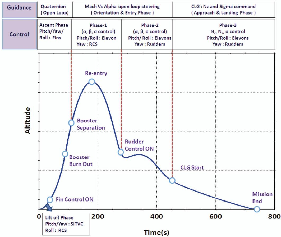
Figure 3. Guidance and control strategies in different phases of the flight.
