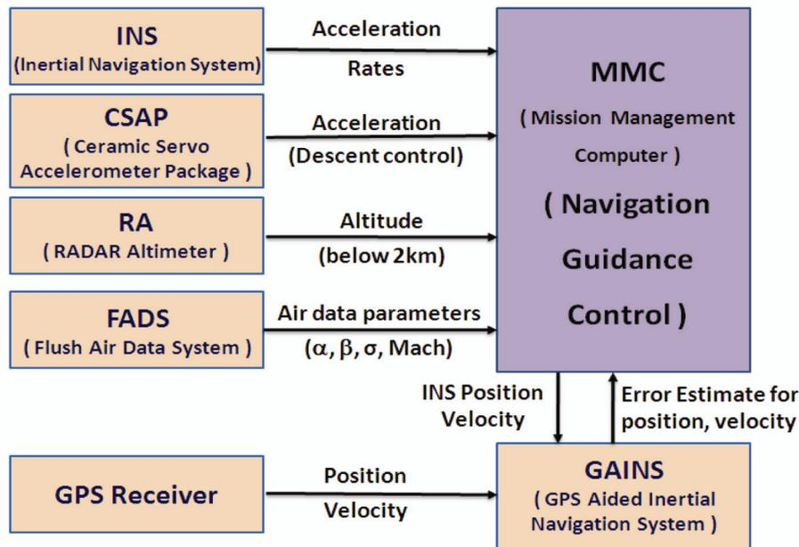
Figure 2. Block schematic of the navigation system.
