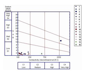
Figure 6. Wilcox diagram of water samples from Kottukal microwatershed during pre-monsoon 2014.
