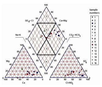
**Figure 5.** Hill–Piper diagram showing different hydrochemical facies of Kottukal microwatershed.
