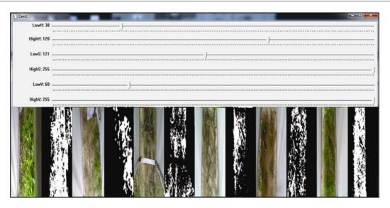
Figure 8. GUI window with original and threshold images during field operation.
