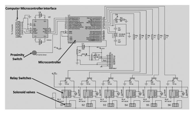
Figure 5. Circuit diagram for the precise herbicide application system.
