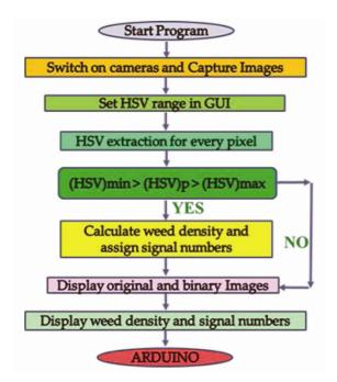
Figure 2. Image analyser process.
