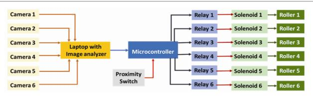
Figure 4. Process flow of the contact-type herbicide application system.
