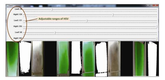
Figure 7. GUI for original and threshold image analysis in laboratory condition with HSV adjustments.
