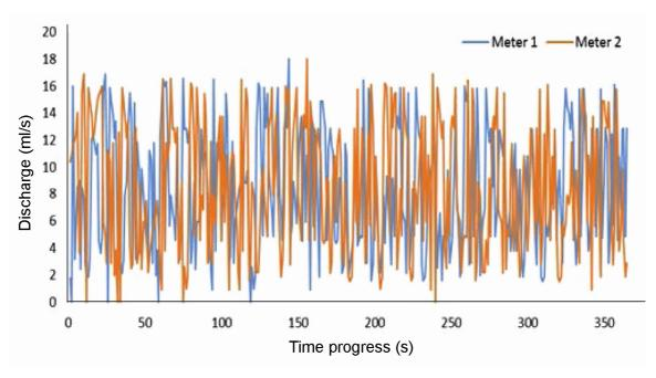
Figure 13. Flow variation recorded by the Hall Effect flow meter per variation in weed density.
