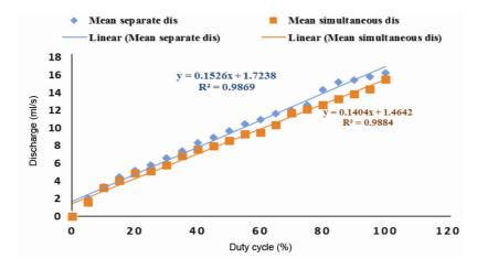
Figure 11. Discharge regression for separate and simultaneous solenoid valve calibration.
