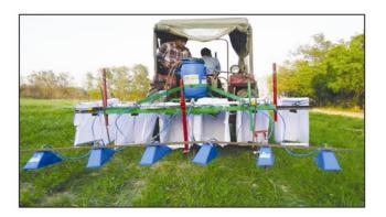
Figure 9. Field evaluation with the spray-type mode of herbicide application.
