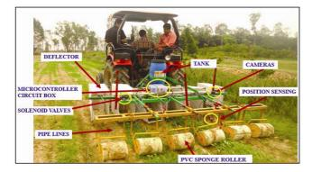
Figure 10. Field tests of the developed variable rate weed eradicator at maize field.
