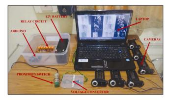
Figure 3. Components of image analysis and controller circuit.
