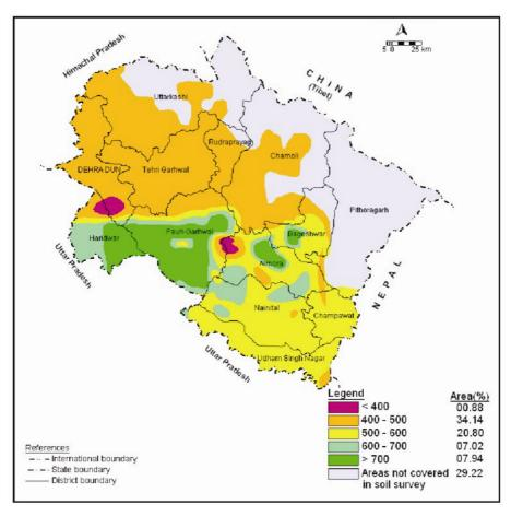
Figure 2. Rainfall erosivity (R-factor) map of Uttarakhand.
