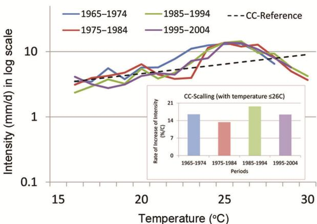
**Figure 2.** The 99th percentile of daily precipitation intensity of wet events ( $\geq 0.05 \text{ mm/d}$ ) as a function of daily mean temperature computed for four decades, viz. 1965–1974, 1975–1984, 1985–1994, and 1995–2004 over India. The inset figure represents the CC-scaling (considering the temperatures  $\leq 26^\circ\text{C}$ ) computed for each decade.
