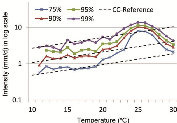
**Figure 1.** Extreme daily precipitation intensities of wet events ( $\geq 0.05 \text{ mm/d}$ ) as a function of daily mean temperature computed from APHRODITE observation for 1961–2007 over India.
