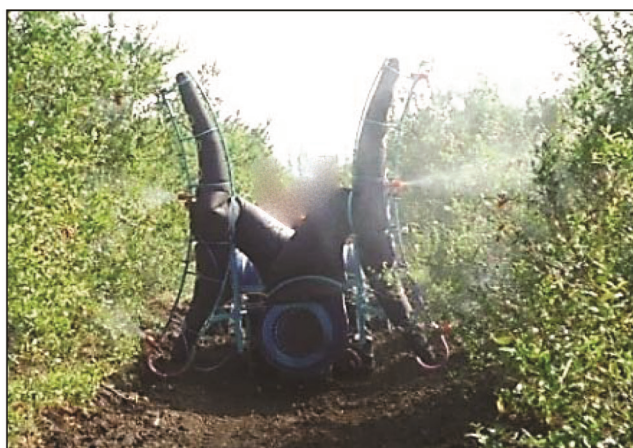
Figure 7. Field tests of the ultrasonic sensor based sprayer in pomegranate orchard.
