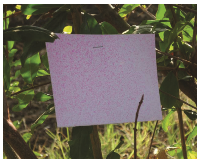
Figure 6. WSP on a pomegranate tree canopy.
