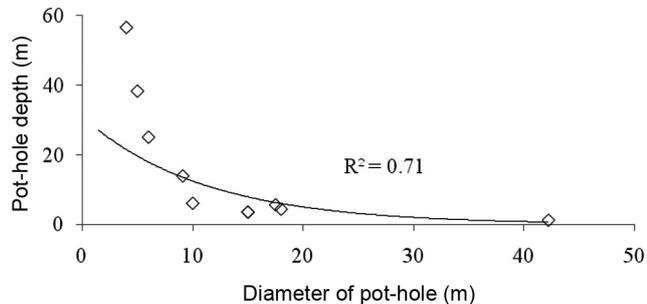
**Figure 7.** Influence of pot-hole diameter on pot-hole depth in Dyne model.
