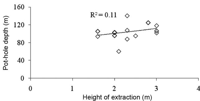
Figure 10. Influence of height of extraction on pot-hole depth of depillaring working in Tajdus and Sroka model.
