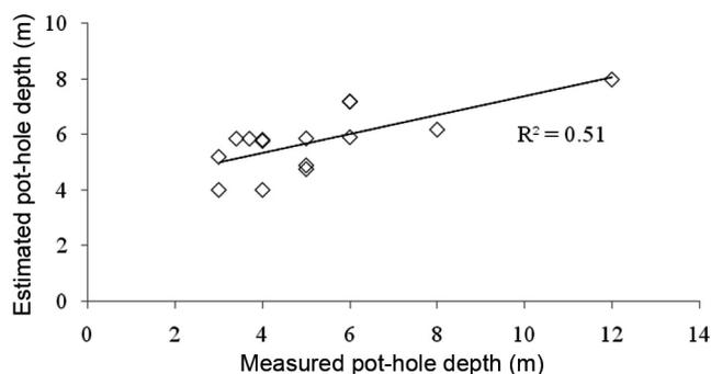
**Figure 14.** Measured and estimated pot-hole depth for depillaring working.
