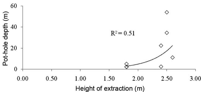
Figure 4. Influence of height of extraction on pot-hole depth in Whittaker and Reddish model.
