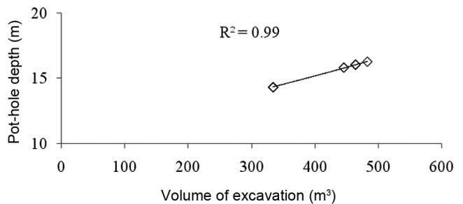
**Figure 9.** Influence of volume of excavation on pot-hole depth of development working in Tajdus and Sroka model.
