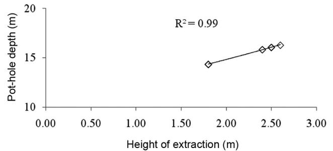
**Figure 8.** Influence of height of extraction on pot-hole depth of development working in Tajdus and Sroka model.
