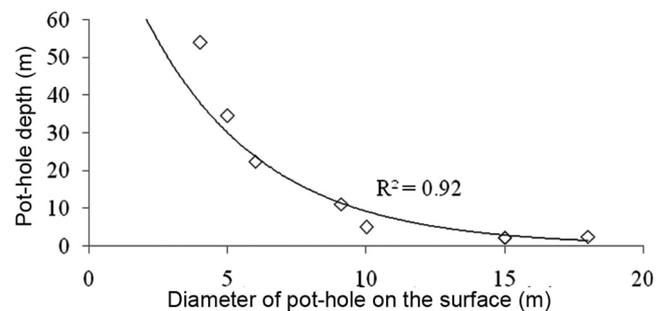
Figure 5. Influence of pot-hole diameter on pot-hole depth in Whittaker and Reddish model.
