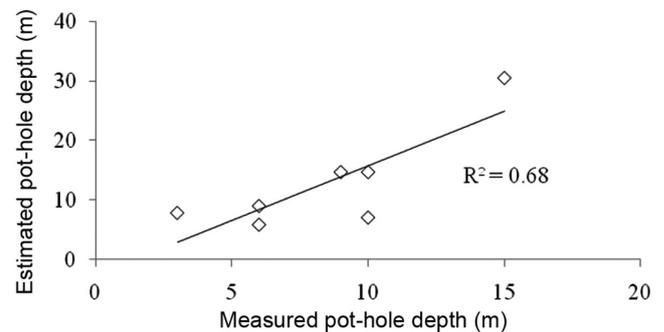
**Figure 13.** Measured and estimated pot-hole depth for development working.
