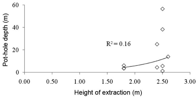
**Figure 6.** Influence of height of extraction on pot-hole depth in Dyne model.
