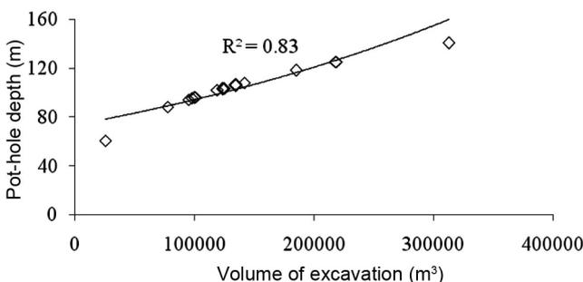
Figure 11. Influence of volume of excavation on pot-hole depth of depillaring working in Tajdus and Sroka model.
