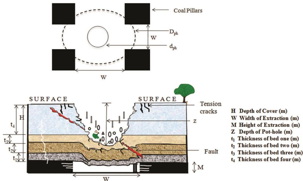
Figure 2. Mechanism of pot-hole subsidence.
