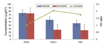
Figure 4. Indoor versus outdoor particulates concentration.
