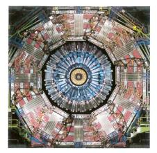
Transverse section of the barrel part of CMS, illustrating the successive layers of detection starting from the centre, where the collisions occur: the inner tracker, the crystal calorimeter, the hardon calorimeter, the superconducting coil, and the iron yoke instrumented with the four muon stations. The last muon station is at a radius of 7.4 m.
