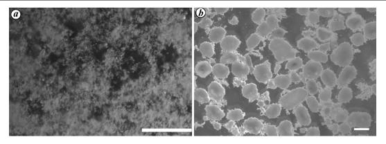
Figure 3. Morphology of (a) activated sludge and (b) aerobic granlar sludge. Scale bar: 1 mm.
