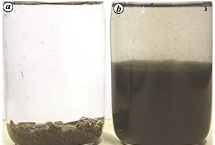
Figure 4. Comparison of volume occupied by equal amounts of (*a*) granular sludge and (*b*) activated sludge after settling.
