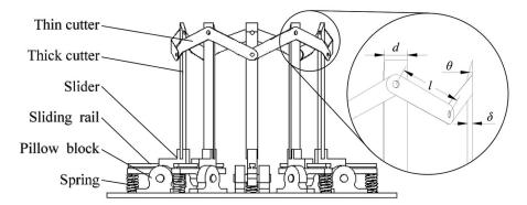
Figure 1. Main mechanical structure of the combined cutting part.
