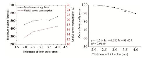
Figure 7. Effect of thickness of thick cutter.
