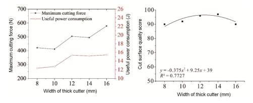
Figure 8. Effect of width of thick cutter.
