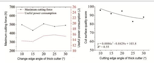
Figure 6. Effect of cutting edge angle of thick cutter.
