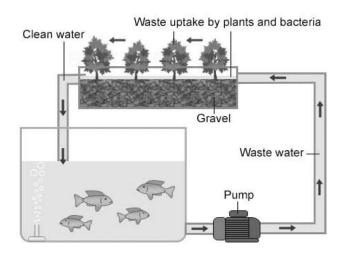
**Figure 3.** Aquaponics system established a co-relationship between soilless cultivation and aquaculture. Water from the water tank in which the fishes are grown is supplied to the plants as nutrition source which returns back after getting filtered.
