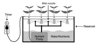
**Figure 2.** The plants in aeroponics system get nutrients from the thin mist formed by the sprayer at the root zone. The timer helps in maintaining the cycle of nutrient supply to the plants so that the roots do not dry up.
