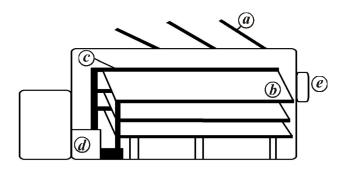
**Figure 4.** Basic design of eco-friendly soilless farming unit (EFSFU). *a*, solar panels; *b*, culture racks; *c*, nutrient supplying system; *d*, control panel; *e*, air circulation system. The front entrance has an extra chamber to keep all sterilized tools, equipments and clothing.
