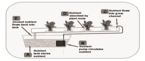
Figure 1. Nutrient film technique is simple yet advanced close soilless system where the plants are supplied with nutrients from the nutrient tank through pump circulation.
