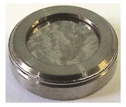
Figure 5. Encapsulated <sup>244</sup>Cm alpha source.
