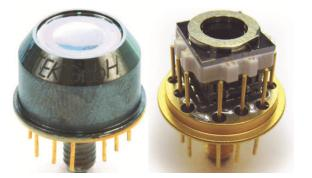
Figure 4. Photographic view of SDD module with and without external cover (Courtesy KETEK, GmbH, Germany).
