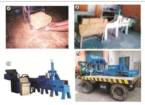
**Figure 2.** *a*, Manually operated feed block-making machine (source: Khan *et al.*<sup>14</sup>). *b*, Power-operated feed block-making machine (Source: Bohra *et al.*<sup>24</sup>). *c*, Electrically powered hydraulic plunger/piston press-type feed block-making machine (source: Bohra *et al.*<sup>24</sup>). *d*, IC engine-operated, tractor trolley-mounted hydraulic plunger/piston press-type feed block-making machine.
