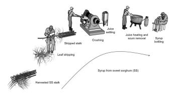
Figure 1. Schematic of the sweet sorghum syrup production process.
