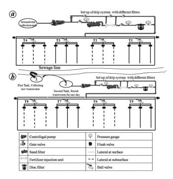
Figure 2. Layout of the experiment under different treatments. a, Groundwater applied for treatments T1 to T4. b, Wastewater applied for treatments T5–T8. Two separate set-ups of drip irrigation system were installed for groundwater and wastewater application.
