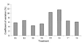
Figure 4. Coefficient of variation of dripper discharge under different treatments.
