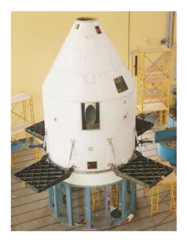
Figure 13. Crew Module Fairing with composite grid fins in deployed condition.
