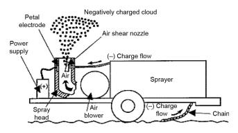
Figure 4. Ionized field charging method (source: ref. 51).
