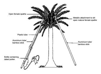
**Figure 1.** Mechanical pollination equipment for date palm (source: ref. 14).
