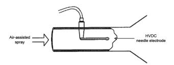
Figure 3. Contact charging method (source: ref. 50).
