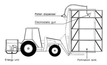
Figure 7. Electrostatic duster for larch (source: ref. 48).
