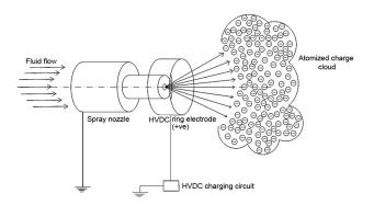
Figure 6. Electrostatic induction charging method (source: ref. 52).
