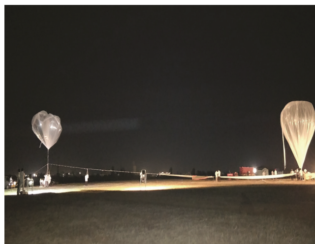
Figure 3. Hydrogen-inflated T500 balloon before lift-off – static anchor line launch method.
