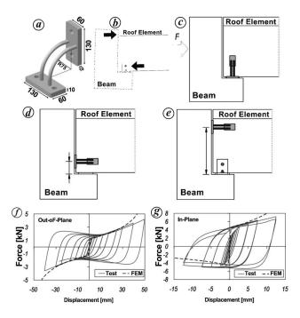
Figure 10. Ductile connection and cyclic test results in terms of load versus displacement (Experimental and Analytical)<sup>64</sup>: a, ASDC details; b, Traditional hinge connection; c, Out-of-plane; d, In-plane; e, In-plane with ASDC and traditional hinge connection; f, Out-of-plane cyclic test result; g, In-plane cyclic test result.
