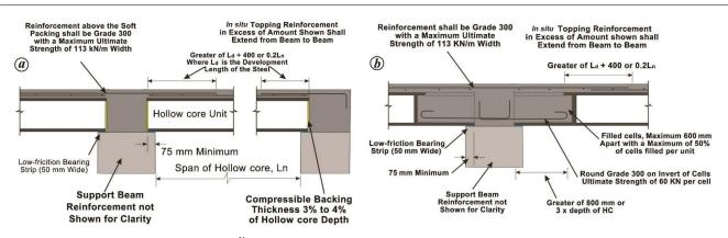
Figure 8. 'Acceptable solution'<sup>51</sup> proposed by New Zealand concrete standards: *a*, First solution; *b*, Second solution.
