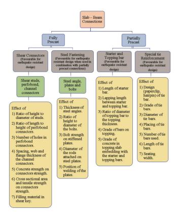
**Figure 1.** Quantitative design parameters influencing the performance of slab to beam connection.
