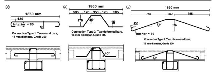
Figure 3. Special tie connection details of test specimen<sup>40</sup>: a, Type 1, Hanger tie; b, Type 2, Saddle tie with 45° bend; c, Type 3, Saddle tie with 13° bend.
