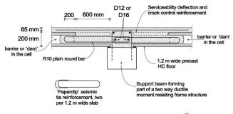
Figure 4. 'Paperclip' tie connection detail<sup>42</sup>.
