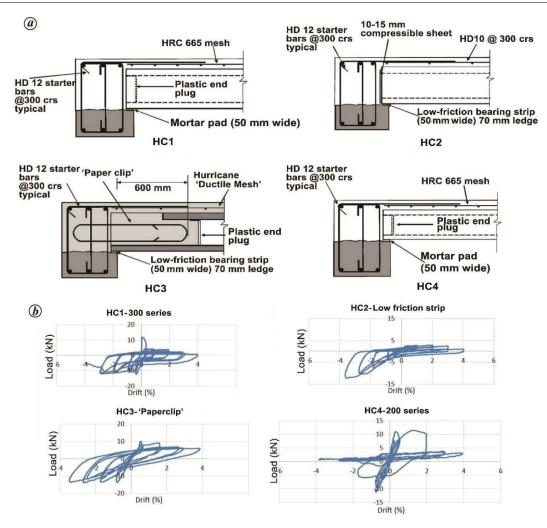
Figure 7. Details of sub-assemblage<sup>46</sup>: a, Connection details; b, Hysteresis performance of the tested connection.
