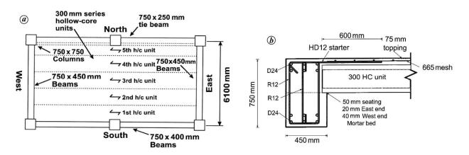
Figure 5. Details of super-assemblage<sup>45</sup>: *a*, Plan; *b*, Connection detail.
