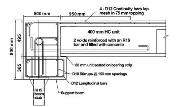
Figure 9. Recommended connection detail for 400 HC from NZS 3101:2006 (ref. 13).
