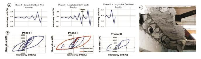
Figure 6. Performance of the super-assemblage test<sup>45</sup>: a, Loading protocol; b, Hysteresis loop; c, Failure mode showing starters and end of the HC units remain attached to the east beam.
