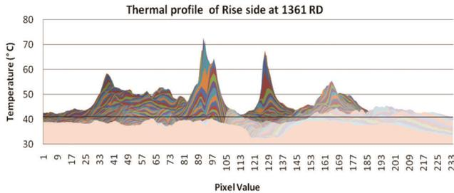
Figure 4. Pixel values assigned for temperatures measured at the rise side of RD 1361 m.
