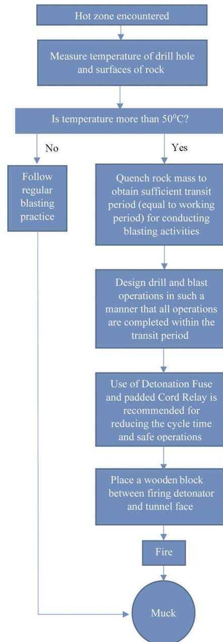
**Figure 9.** Methodology for blasting hot zone in tunnels.
