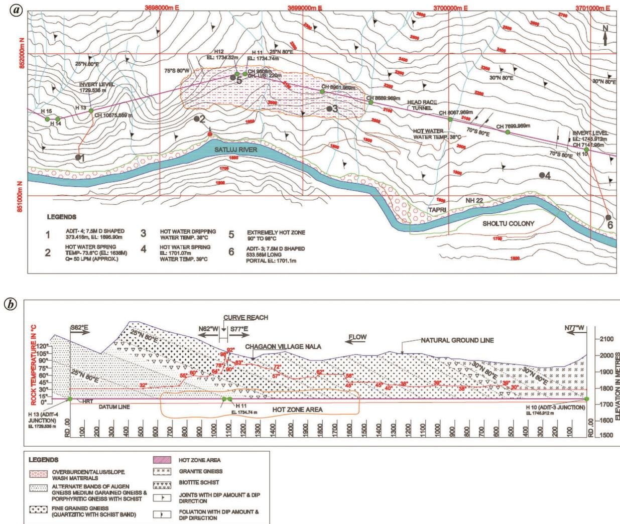
**Figure 2.** a, Topographical layout of the hot zone and its surrounding area. b, Geological cross-section of head race tunnel.
