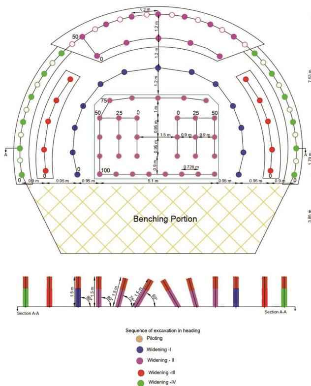
**Figure 7.** Sequence of excavation and blast design for temperatures greater than 70°C.
