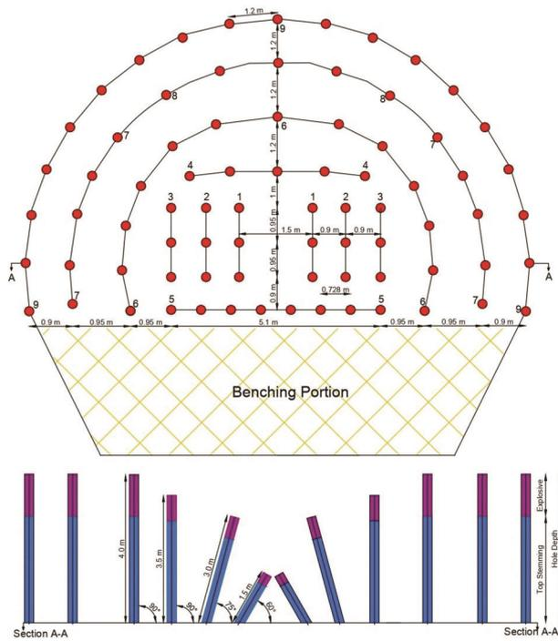
Figure 6. Initial excavation sequence.
