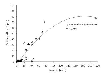
**Figure 9.** Relationship between long-term (1986–2000) observed soil loss and run-off under jhum cultivation from two hill districts of Assam (Karbi Anglong and North Cachar Hills) (modified from Baruah *et al.*<sup>25</sup>).
