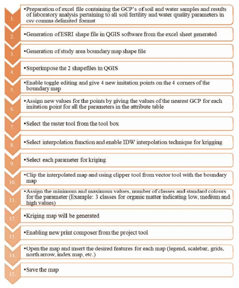
Figure 1. Generation of soil fertility maps using kriging and interpolation.
