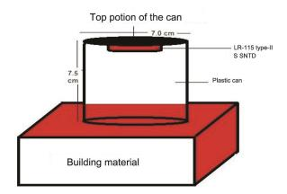
Figure 2. Measurement of radon exhalation rate using the 'can technique II'.
