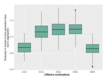
**Figure 7.** Reduction in fraction of zero generation days in 1000 years due to aggregation of different combinations of four wind plants from different boxes (A and B). Combination of plants from different regions demonstrates larger reduction in fraction of 'no generation' days by aggregation of generation.
