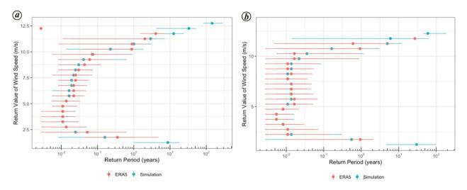
**Figure 5.** Return period (*x*-axis) of daily average wind speed (*y*-axis) over (*a*) Rajasthan and (*b*) South India from ERA5 reanalysis and IMAGE simulations. The points indicate the median return periods, while horizontal lines show the distribution of return periods.
