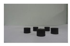
Figure 11. B4C pellets. CURRENT SCIENCE, VOL. 123, NO. 3, 10 AUGUST 2022
