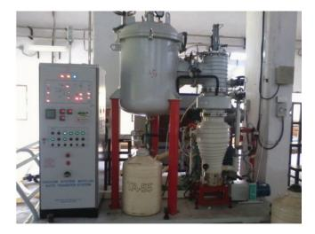
Figure 10. High vacuum induction furnace.
