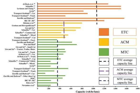
Figure 5. Capacity from literature for a different type of toll collection systems.
