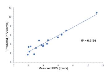
Figure 4. Relation between predicted and measured peak particle velocity using ANN.
