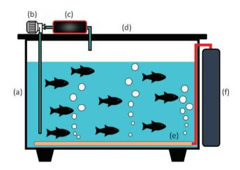
**Figure 1.** Schematic representation of closed system for live fish transportation. a, Container; b, pump; c, filtration unit; d, lid; e, oxygen diffuser; f, in-built oxygen source.
