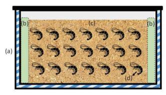
Figure 3. Schematic representation of waterless system for live fish transportation. a, Insulated container with lid; b, cooling unit; c, pre-chilled layering medium; d, live fish/shellfish.
