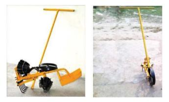
**Figure 2.** The weeder with a single front wheel and addition of conical rotors and boat for operation in transplanted rice (from left).
