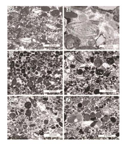
**Figure 2.** Photomicrographs of different varieties of carbonate aeolianite. *a*, Typical biopelsparite; *b*, well-rounded clast of foraminifera; *c*, typical pelsparite; *d*, *e*, pelbiosparite; *f*, pelsparite<sup>34</sup>.
