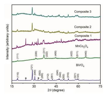
**Figure 1.** Powder XRD patterns of as-prepared  $BiVO_4$ ,  $MnCo_2O_4$  and their composites (\* indicates peaks from secondary tetragonal  $BiVO_4$  phase).
