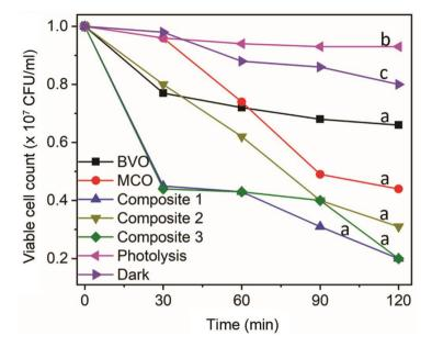
Figure 5. Plot of viable cell count vs time indicating the inactivation of *E. coli* as a function of time: (a) as-prepared compounds, (b) photolysis (with light and without composite) and (c) dark experiment (without light and with composite).
