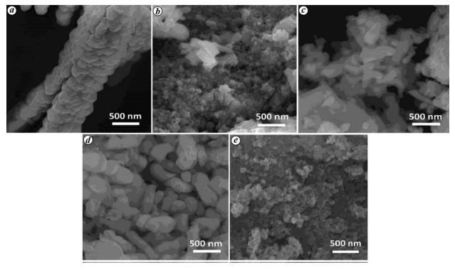
**Figure 3.** SEM images of as-prepared BiVO<sub>4</sub>,  $MnCo_2O_4$  and their composites. (*a*) BiVO<sub>4</sub>, (*b*) composite 1, (*c*) composite 2, (*d*) composite 3 and (*e*)  $MnCo_2O_4$ .
