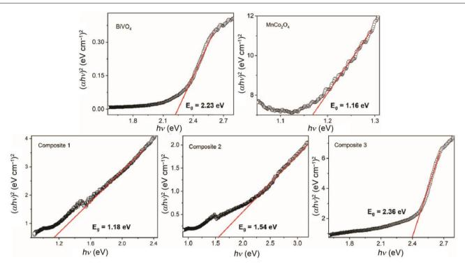
Figure 2. Tauc plots to determine band gaps of all the as-prepared compounds estimated using absorption data from diffuse reflectance spectra.
