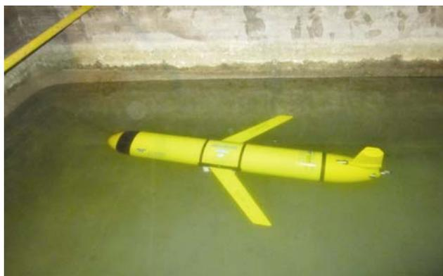
**Figure 3.** A properly ballasted glider for tank water.
