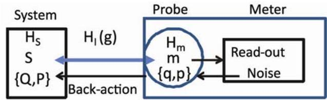
**Figure 1.** Scheme of a quantum measurement. See text for details. The final stage of coupling a classical meter to the probe involves collapse of the state as well as injection of quantum and other sources of noise back into the probe system. A proper choice of the probe observable avoids back-action on the signal.
