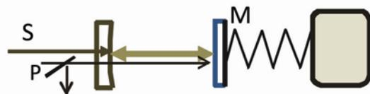
**Figure 2.** Radiation pressure of the signal beam (S) causes fluctuations in the position of the mirror on spring (M) and in turn changes the phase of the resonant weak probe beam (P) in the cavity configuration.
