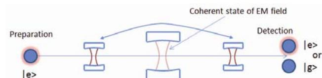
**Figure 4.** QND–BAE measurement of the number of microwave quanta in the cavity. The central cavity has a small number of photons that change the relative phase of the superposition of the excited and ground states of the passing atoms. The two auxiliary cavities define a Ramsey interferometer with a scannable relative phase. Final state selective detection enables an iterative determination of the number state inside the main cavity. See text for more details.
