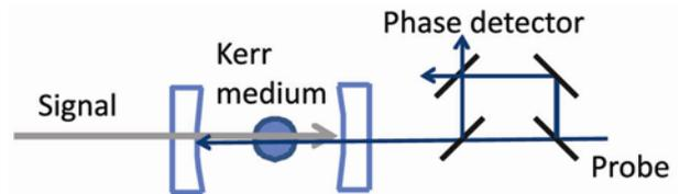
**Figure 3.** Schematic diagram of an optical QNDM. The strong signal and weak probe beams interact via a Kerr nonlinearity in the atomic medium, causing a change in the phase of the probe proportional to the intensity of the signal. Intensity of the signal beam is not affected by the increased uncertainty in the amplitude quadrature of the probe because the precision phase measurement changes only the phase of the signal and not its amplitude, enabling back-action evasion.
